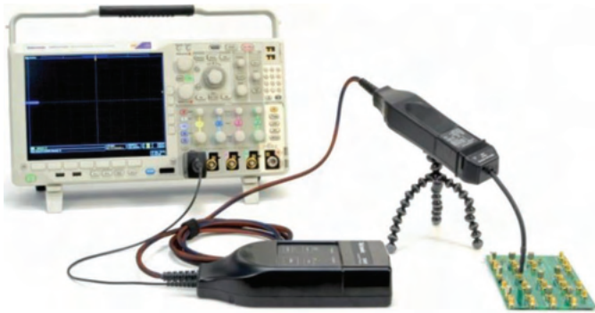
Figure 4: Tektronix IsoVu measurement setup.
