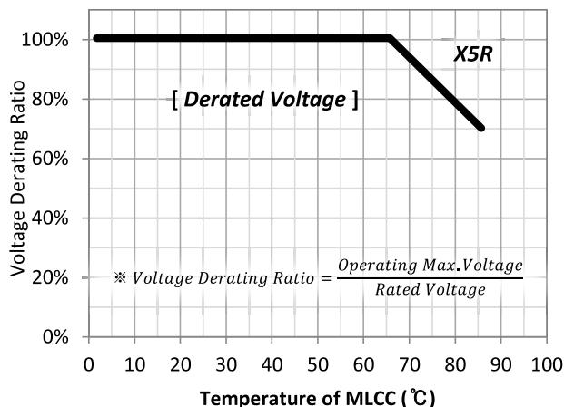
\* Temperature of MLCC : Surface temperature of MLCC in the circuit.
