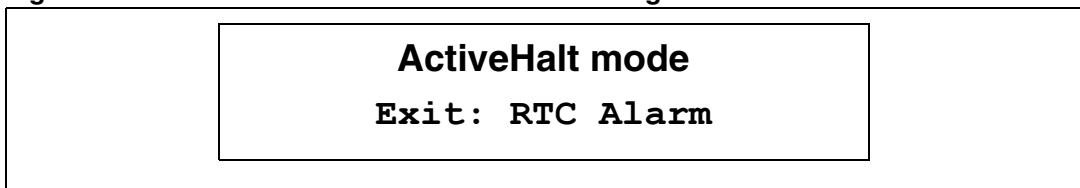
Figure 31. Exit from Active-halt with alarm message
