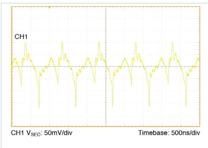
Figure 14 — Full load ripple, 10\mu\text{F} C_{PRI\_IN\_EXT} ; No external C_{SEC\_OUT\_EXT} . Board mounted module, scope setting: 20MHz analog BW
