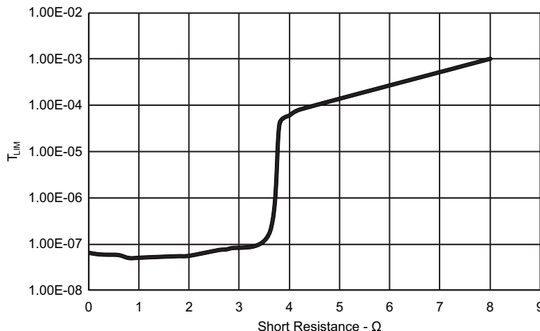
Figure 8. Overcurrent Response Time vs Short Resistance
