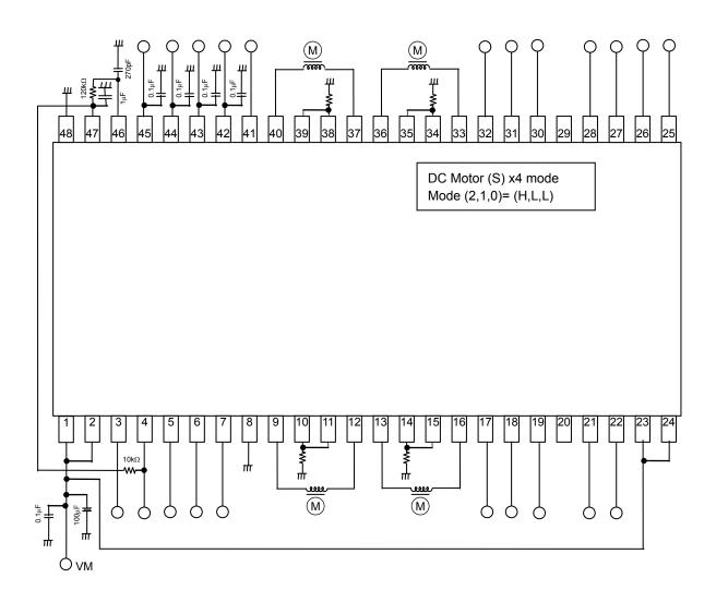
Note: It is recommended that a bypass capacitor is added if necessary. The GND wiring must become one-point-earth as much as possible.
