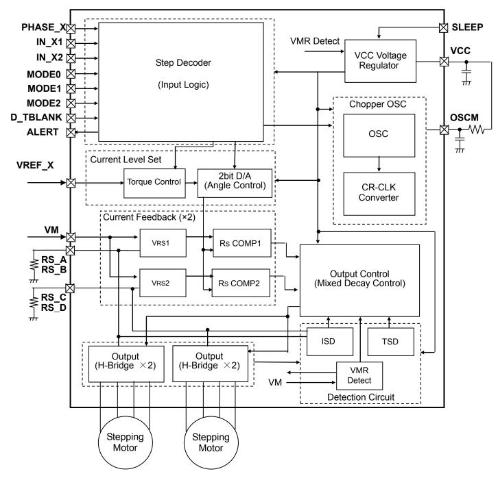
\*: "X" means the ellipsis of A / B / C / D of each Ch. (PHASE\_X, IN\_X1/X2, and VREF\_X)
