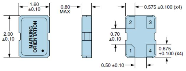
Seam Sealed Terminal Plating Thickness: Gold (0.3 to 1.0µm) over Nickel (1.27 to 8.89µm).
