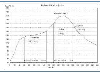
• Preheating shall be fixed at 150~180°C for 60~90 seconds.
