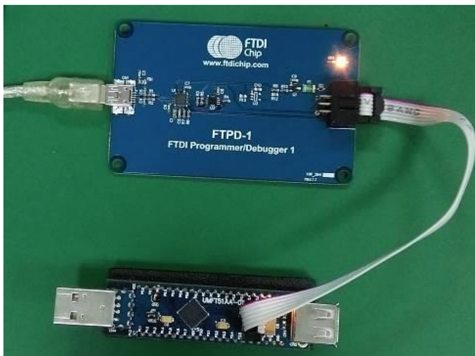
Figure 5 - FTPD-1 connection to UMFT51AA-1
