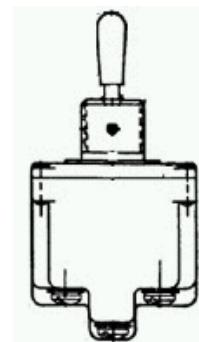
**TL Series Toggle Switch, 4 pole, 3 position, Screw terminal, Standard Lever**
