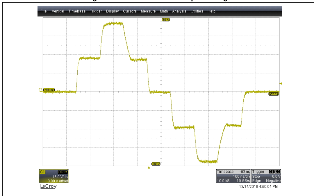
Figure 14. Five-levels HV output voltage
