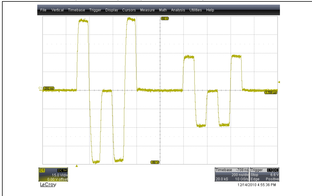
Figure 13. TX0 = \pm 60 V positive-negative pulses and immediately after TX1 = \pm 30 V positive-negative pulses, load 300 pF // 100 \Omega
