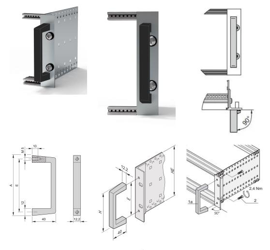
The handle can be assembled to a subrack or 19" front panel. Available with clear or black anodized surface. Handles will be bolted from the rear side.
