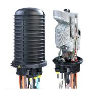
FIST™ GCO2 Fiber Optic Splice Closure, Heat Shrink Cable sealing, size BE, no pre-installed fiber trays, 6 ports, with test valve
