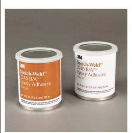
3M™ Scotch-Weld™ Epoxy Adhesive 2216 is a flexible, two-part epoxy adhesive. 1:1 mix ratio, 120 minute work life and handling strength in approximately 10 hours. This kit contains 1 pint of part B and 1 pint of part A.
