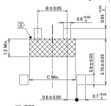
Note: 2 If there is a pattern on the area and resist is not applied, it may come into contact with the connector terminal.
