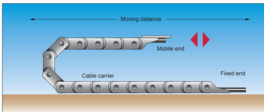
Cable carrier bending radius: approx. 9 x cable outer diameter
