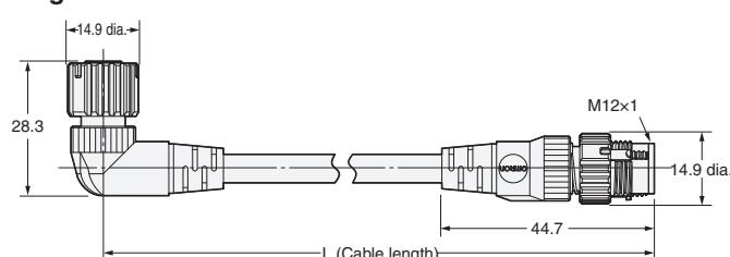
**Note:** Oil-resistant Polyurethane Cables (XS5W-D42□-□81-P) and Spatter-resistant Cable (XS5W-D421-□81-SA) have black covers.
