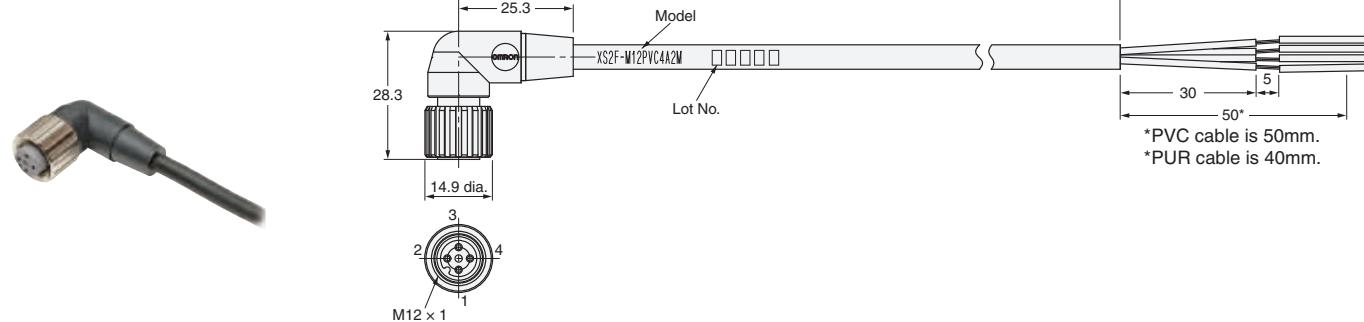
Note: For 3-core, pin 2 is not connected internally
