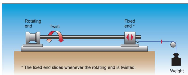
Torsion angle and length: PVC:  $\pm 180^\circ$  over 0.5 m
