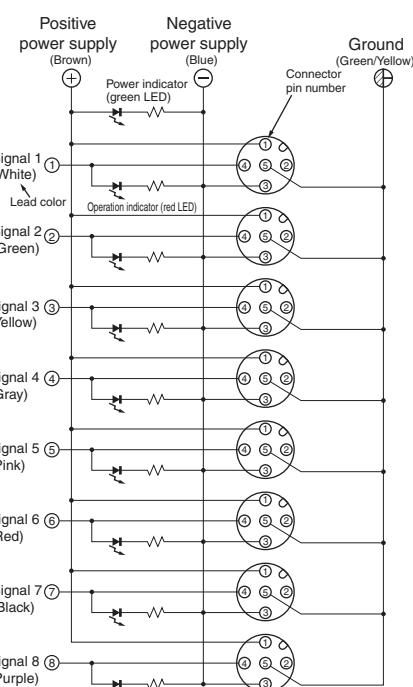
Note 1. The above wiring diagrams are for eight-port use.
