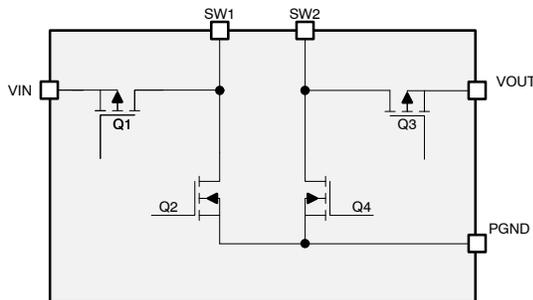
Figure 29. Simplified Block Diagram
