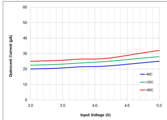
Figure 7. Quiescent Current (No Switching) vs. Input Voltage
