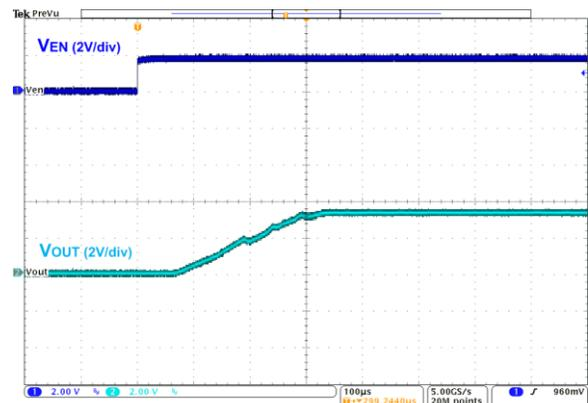
Figure 27. Startup, VIN = 3.6 V,  $I_{OUT} = 1000\text{ mA}$
