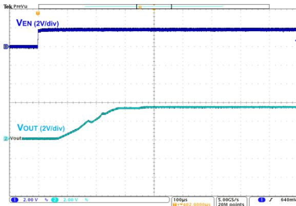
Figure 26. Startup, VIN = 3.6 V,  $I_{OUT} = 68\text{ mA}$
