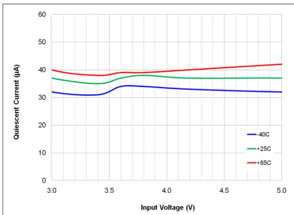
Figure 8. Quiescent Current (Switching) vs. Input Voltage
