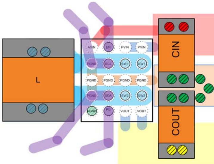
Figure 30. Component Placement and Routing for FAN49100
