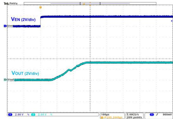
Figure 25. Startup, VIN = 3.6 V,  $I_{OUT} = 0\text{ mA}$
