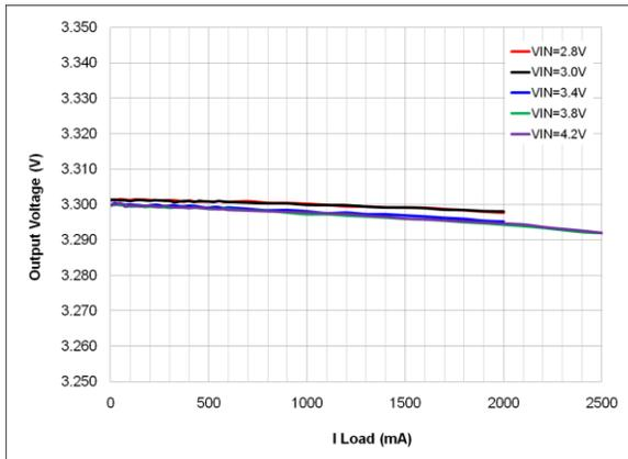
Figure 6. Output Regulation vs. Load, PWM Mode
