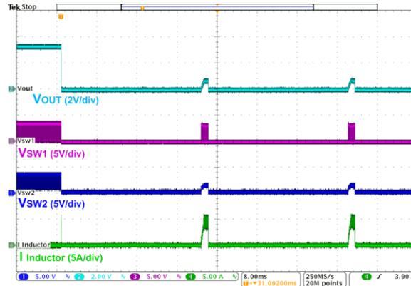
Figure 28. Short-Circuit Protection
