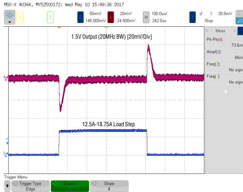
Figure 5. Measured Channel 1 12.5A-18.75A Load Transient ( V_{IN} = 12V , V_{OUT1} = 1.5V )
