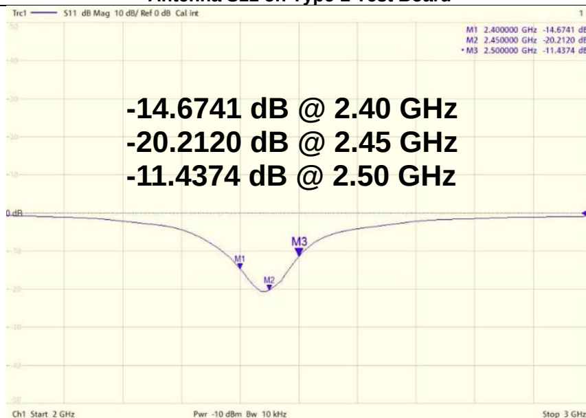
Antenna VSWR on Type-2 Test Board
