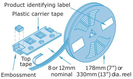
Tape and reel packing of surface mounting chip capacitors for automatic placement are in accordance with IEC60286-3.
