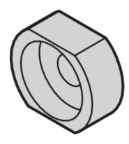
Sleeve guides the collar screw when fastening the front panel.
