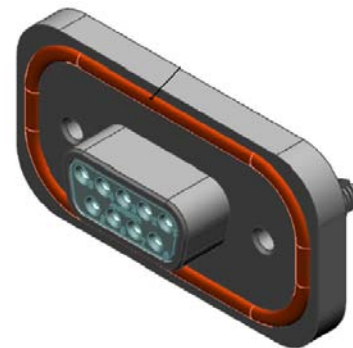
P/N MDB-E09SE-860 SHOWN 9 POSITION SOCKET, VERTICAL PCB TAILS WITH BOARDLOCK
