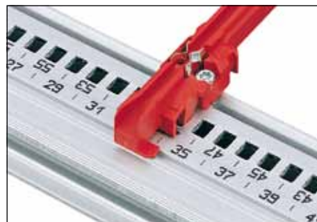
Continuous numbering on the profile rails and a punching, with marking in the card guide, provide a fast visual guide to insertion. The card guides can be screwed into position for extra stability. Card earthing springs at the front and back protect the electronics against electrostatic discharging.
