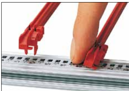
All guide rails have stable snap-in fixings to ensure a firm fit. Tip to the side for easy unlocking. Various card guides are available for the use of coding pegs and card retainers.
