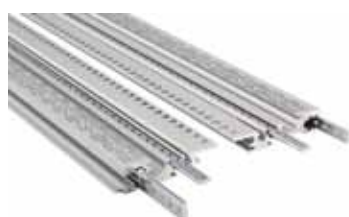
Tapped stripe, galvanised steel, M2.5, 5 x 1.5 mm, for horizontal profile grooves and rear fixing of backplanes, insulating strips and Z rails
