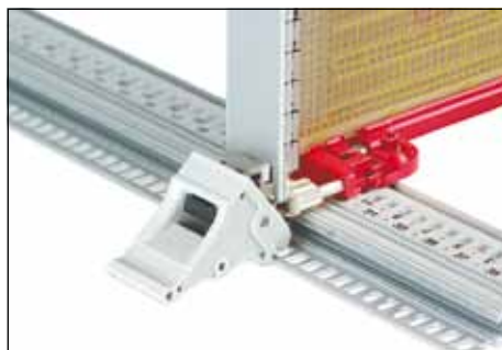
Plug-in units with HGS handle for insertion and withdrawal function comply with standards DIN IEC 60297-3-102/IEEE 1101.10. Optimal leverage effect overcomes high insertion and withdrawal forces.
