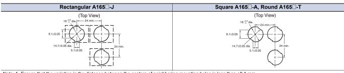
Note: 1. Ensure that the variation in the distance between the centers of neighboring mounting holes is less than ±0.1 mm. 2. Make sure the thickness of the mounting panel is 0.5 to 3.2 mm. If, however, a Switch Guard or Dust Cover is used, the thickness of the mounting panel must be 0.5 to 2 mm.
