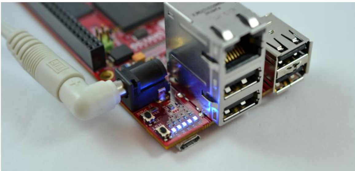
Figure 6: OSD3358-SM-RED Board Boot - LEDs D4 - D7 turn ON
