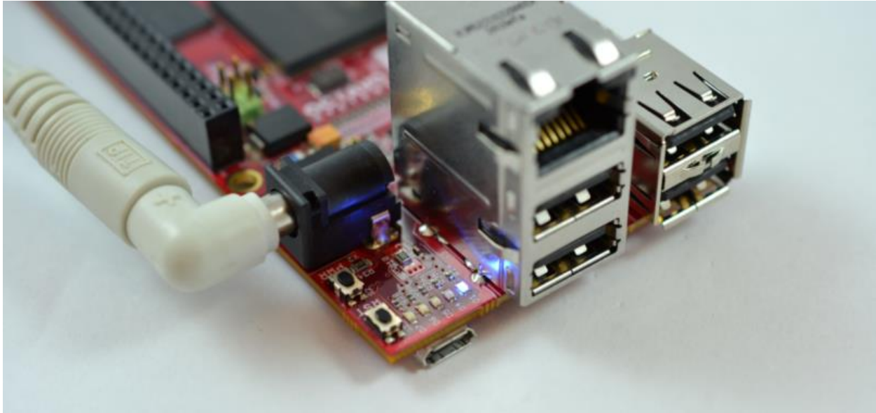
Figure 3: Powering the Board using an AC-DC Adapter
