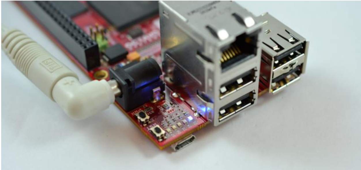
Figure 10: AC-DC Adapter Plugged in to the Board
