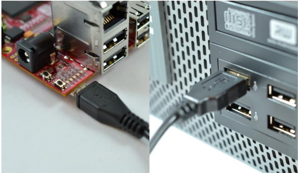
Figure 2: Powering the Board using a USB Cable
