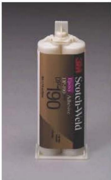
3M™ Scotch-Weld™ Epoxy Adhesive DP190 is a gray, two-part epoxy adhesive. 1:1 mix ratio, 90 minute work life and handling strength in approximately 10 hours. 3M™ Scotch-Weld™ EPX™ Plus II applicator and mix nozzles are required for dispensing (not included).
