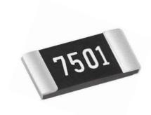
TE are pleased to introduce the new 3504 series. This is a high stability Thin Film Chip Power resistor range offering very high power / size ratio -6W in 2512 size. The 3504 series offers TCR at  $\pm 50$ ppm/°C and resistance tolerance at  $\pm 1\%$  as standard. Resistance values are within the IEC 63 E96 and E24 value grids. The 3504 resistors have accurate and uniform physical dimensions to facilitate automatic placement methods.
