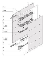
Carrier Mechanics for Mezzanine Module, Stainless steel (EMC shielded).
