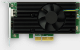
Mustang-V100-MX4 4 x Intel® Movidius™ Myriad™ X MA2485 VPU Accelerator
