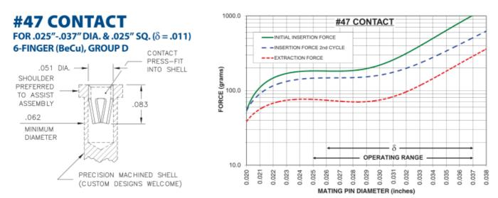
The insertion / extraction force characteristics above were derived using a 30 microinch gold-plated contact and polished steel gauge pins having a bullet-shaped tip. The curves represent typical average values; they are best used to compare the differences between similar size contacts and to guide you in selecting one that is suitable for your application. Your results may vary, so for your specification, we encourage you to obtain complimentary samples for your evaluation.
