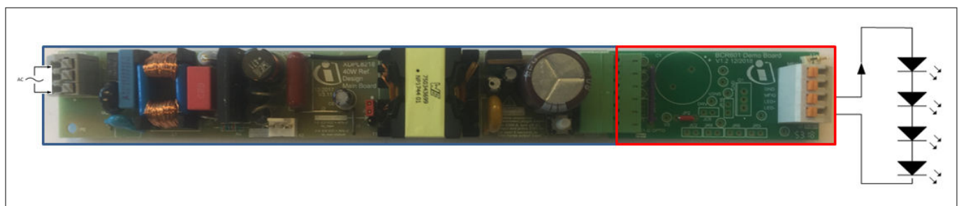
Figure 7 XDPL8218 BCR601 system - top side
