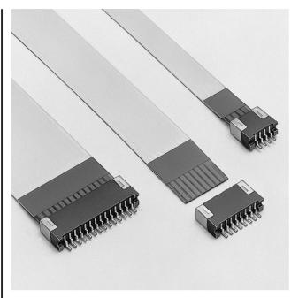
The FMS series connectors are designed for surface mounting (SMT) and to meet the demand for high-density packaging. They are miniature connectors with a height of only 2.8mm, and can be supplied packaged in embossed tape to facilitate automatic mounting.
