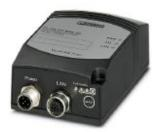
WLAN Ethernet port adapter, client, WLAN 802.11 a/n, 5.15 ... 5.25 GHz frequency, IP65, connections: M12 for 9 ... 30 V DC, M12 for LAN, autocrossing, PROFINET and PROFIsafe-compatible, web-based management, 802.11i, WPA2, WPA-PSK, WEP, TKIP, AES, integrated antenna
