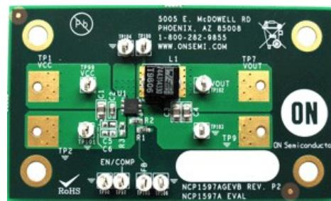
Other features include cycle-by-cycle current limiting; short-circuit protection, power saving mode and thermal shutdown.
