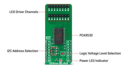
Any bits not used for controlling the LED channels can be used for General Purpose parallel Input/Output (GPIO) expansion, providing a simple solution when additional I/O is needed for some power switches, sensors, push-buttons, alarm monitoring, fans, or other applications.
