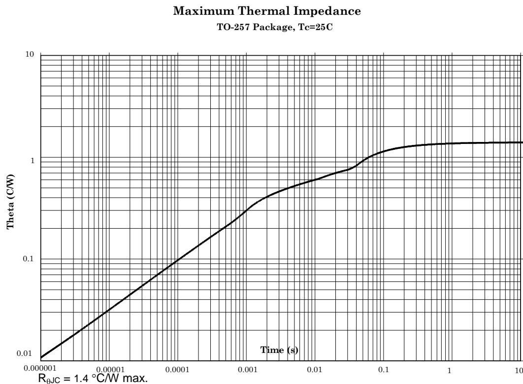
FIGURE 8. Thermal impedance graph (2N6546T3 and 2N6547T3).
