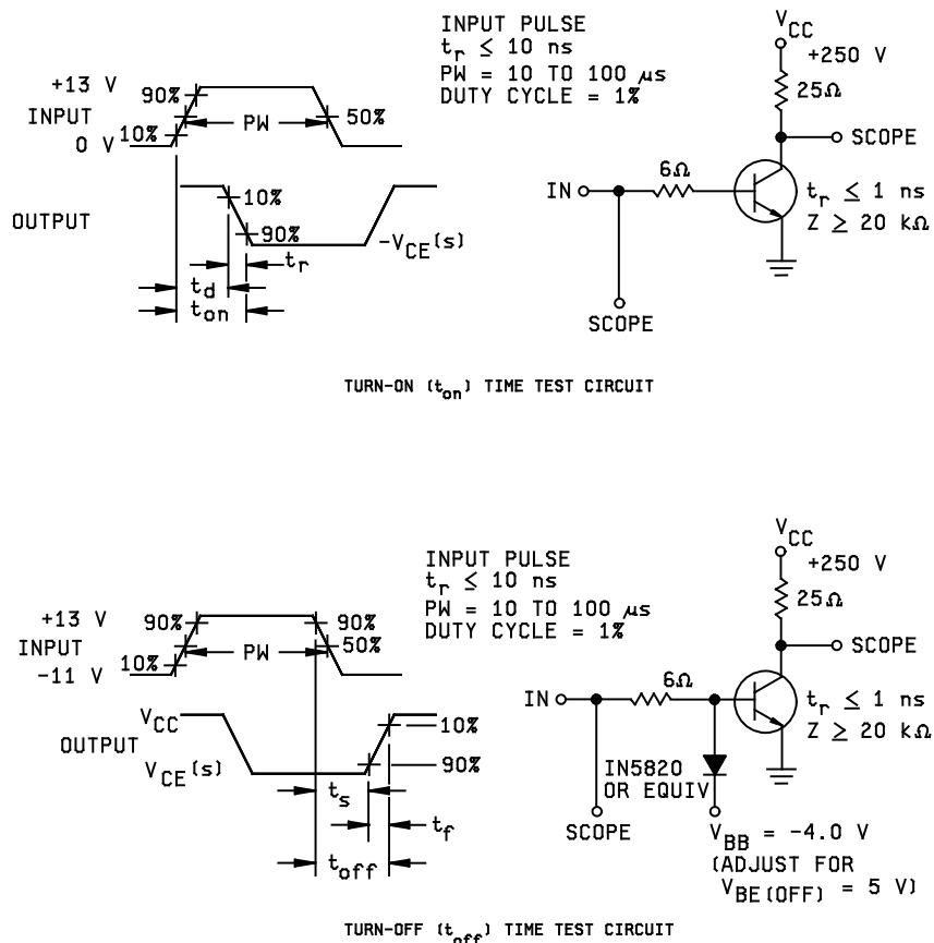
FIGURE 9. Switching time test circuits.
