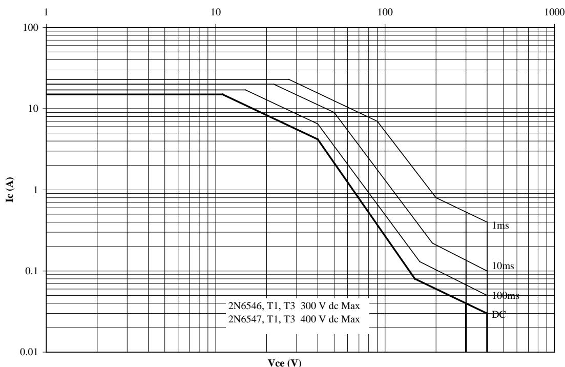
FIGURE 10. Maximum safe operating area graph (continuous dc).
