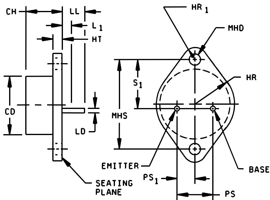
FIGURE 1. Dimensions and configuration (TO-3).
