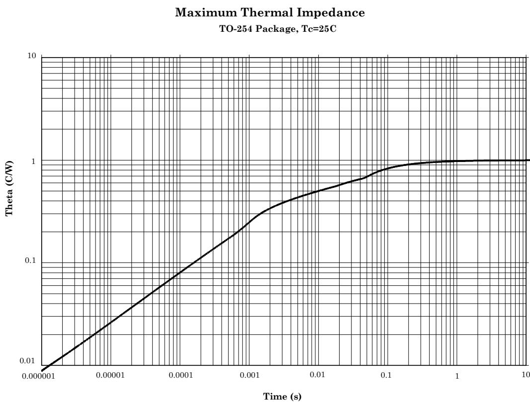
FIGURE 7. Thermal impedance graph (2N6546T1 and 2N6547T1).
