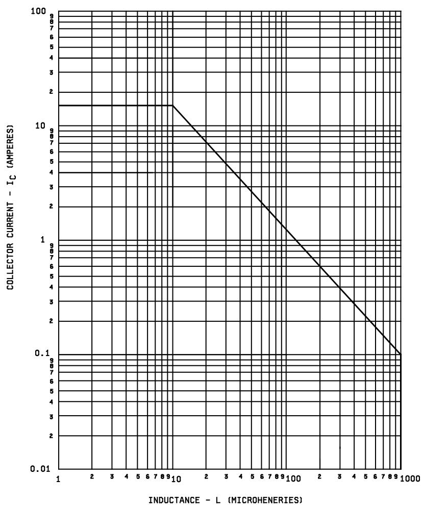
FIGURE 11. Safe operating area for switching between saturation and cutoff (unclamped inductive load, all devices).
