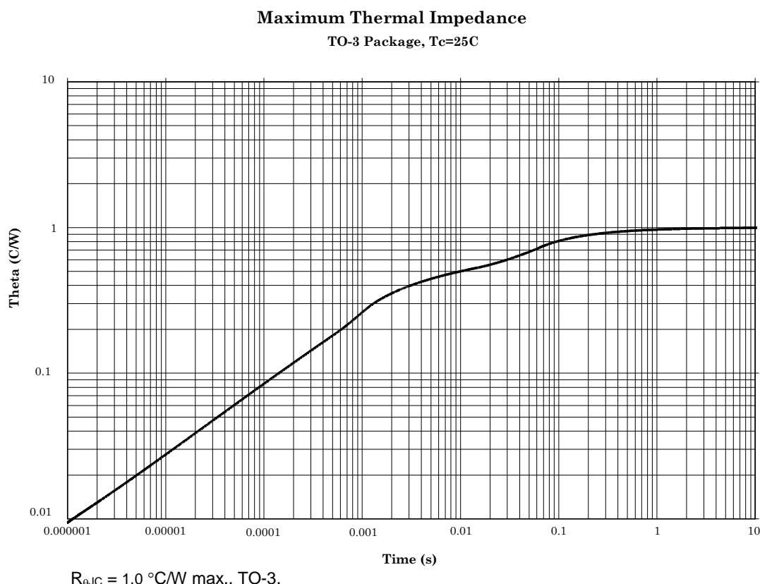
FIGURE 6. Thermal impedance graph (2N6546 and 2N6547).
