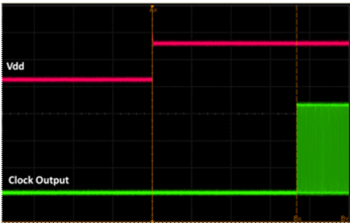
Figure 16. Startup Waveform vs. Vdd
