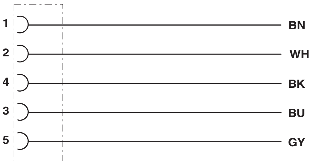
Contact assignment of the M12 socket
