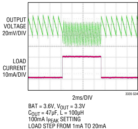
Buck-Boost Load Step Transient
