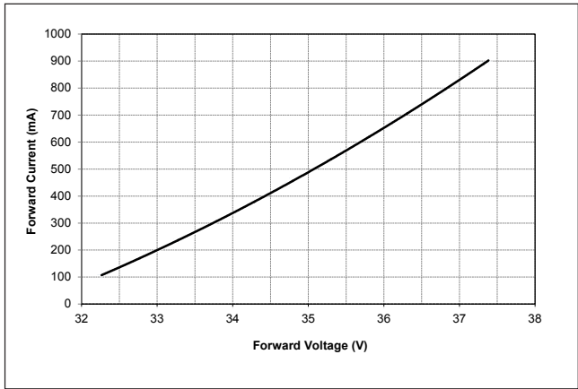
Figure 1: V13B Drive Current vs. Voltage
