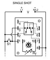
2-3 & 7-6 are Normally Open Contacts (NO) 2-4 & 7-5 are Normally Closed Contacts (NC)
