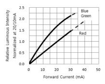
Fig. 4 RELATIVE LUMIOUS INTENSITY VS. FORWARD CURRENT
