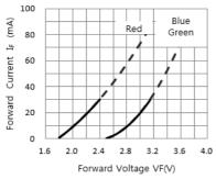
Fig. 2 FORWARD CURRENT VS. FORWARD VOLTAGE
