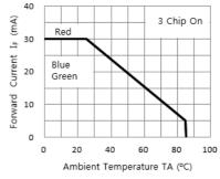
Fig. 3 FORWARD CURRENT VS. DERATING CURVE
