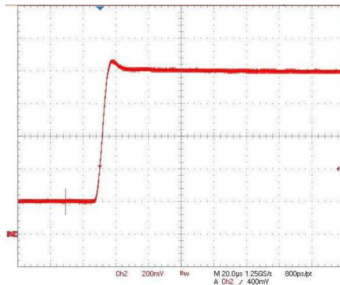
Figure 75. Loop Current Step From 4 mA to 20 mA
