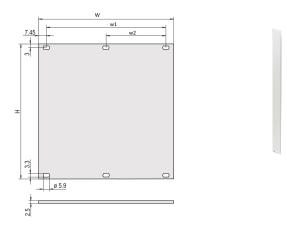
Front panel, unshielded, front anodized and rear conductive.
