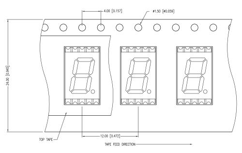
\*UNLESS OTHERWISE SPECIFIED TOLERANCES PER DECIMAL PRECISION ARE: X=±1 (±0.039), X.X=±0.5 (±0.020), X.XX=±0.25 (±0.010), X.XXX=±0.127 (±0.005). LEAD SIZE=±0.05 (±0.002), LEAD LENGTH=±0.75 (±0.030). MIN=  $^{+0.00}_{-0.00}$  MAX.=  $^{+0.00}_{-0.00}$ UNCONTROLLED DOCUMENT
