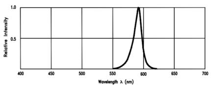
Fig.1 Relative Intensity vs. Wavelength
