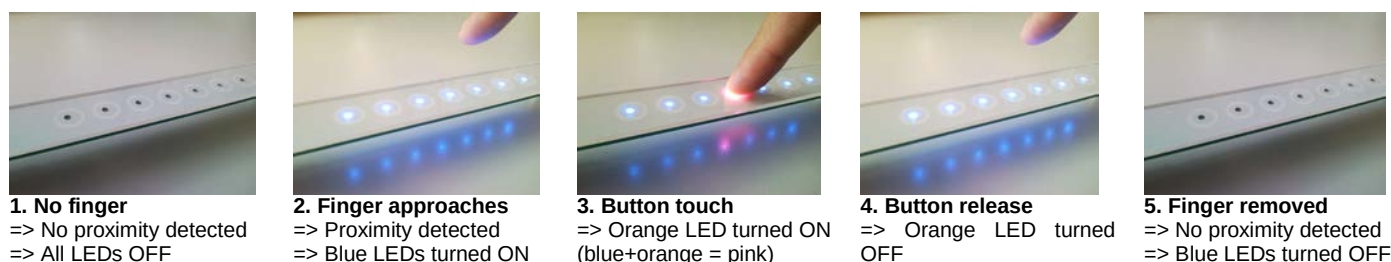
Figure 52 Touch+Proximity Module Operation
