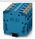
High-current terminal block, nom. voltage: 1500 VDC / 1000 VAC, nominal current: 309 A, connection method: Power-Turn connection, number of connections: 2, number of positions: 1, cross section: 50 mm<sup>2</sup> - 150 mm<sup>2</sup>, AWG: 1/0 - 300 kcmil, width: 31 mm, color: blue, mounting type: NS 35/15
