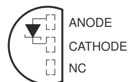
1.2 V . . . LP (TO-92/TO-226) PACKAGE (TOP VIEW)
