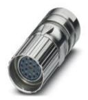
Cable connector, straight, shielded: yes, Screw locking, M23, Number of positions: 16+2+PE, Type of contact: Socket, Crimp connection, Cable diameter: 3 mm ... 14.5 mm
